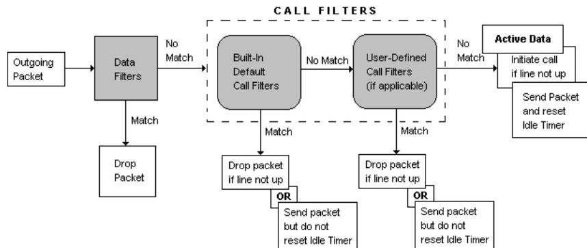
Figure 10-1 Outgoing packet filtering Process
