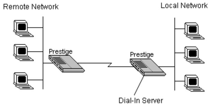
**Figure 6-2 Example of a Dial-In Server Application**
