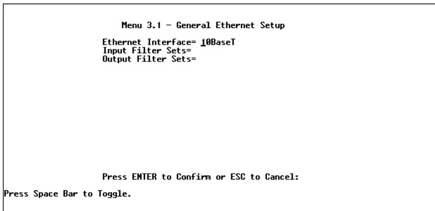
**Figure 3-11 Menu 3.1 - General Ethernet Setup**
