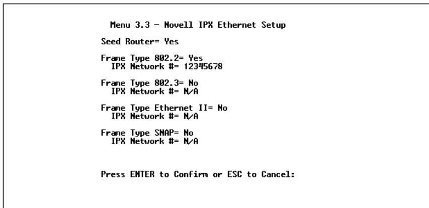
**Figure 8-2 Menu 3.3 - Novell IPX Ethernet Setup**
