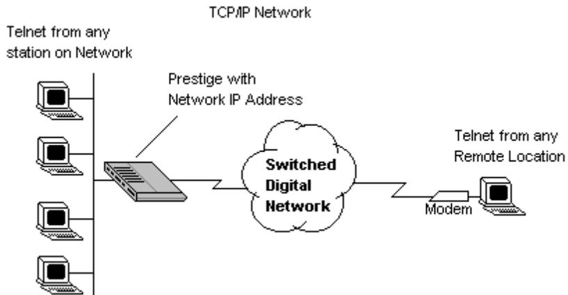
**Figure 13-1 Telnet Configuration on a TCP/IP Network**
