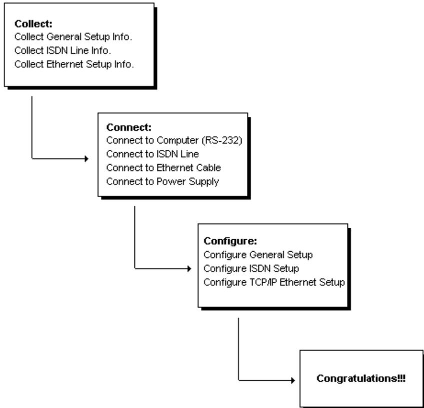
Figure 2-1 Installation Guide
