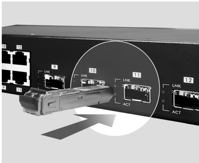
Figure 3-2 Transceiver Installation Example
