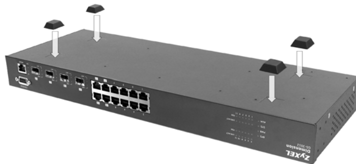
Figure 2-1 Attaching Rubber Feet
