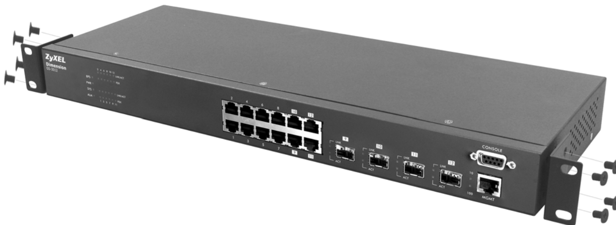
Figure 2-2 Attaching Mounting Brackets and Screws
