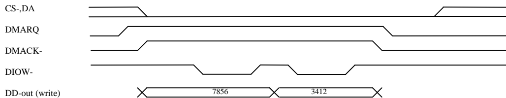
Figure 4.8 32bit DMA write transfer, with endian conversion
