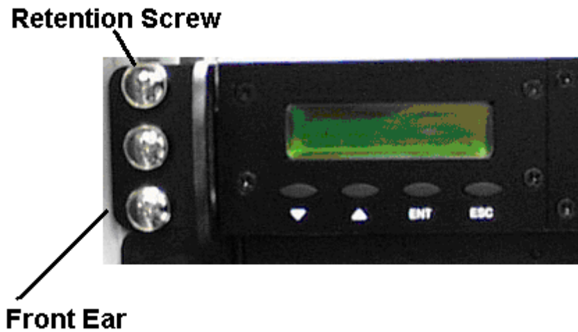
Figure 2-20: Firmly secure the front ears to the sides of the cabinet
