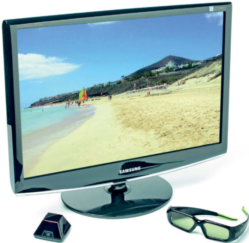
The Nvidia 3D Vision system (shown here with a compatible Samsung monitor) has become the de facto standard for 3D computer imaging. The system's active shutter glasses are synchronized using a separate USB transmitter.
