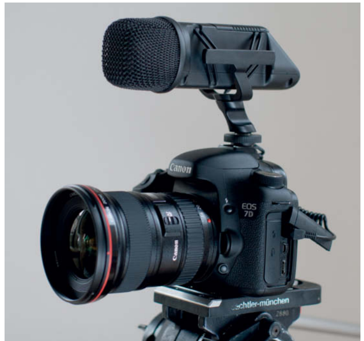
A purpose-built stereo microphone such as this shock-mounted Røde model provides much better sound than the camera's built-in microphone
