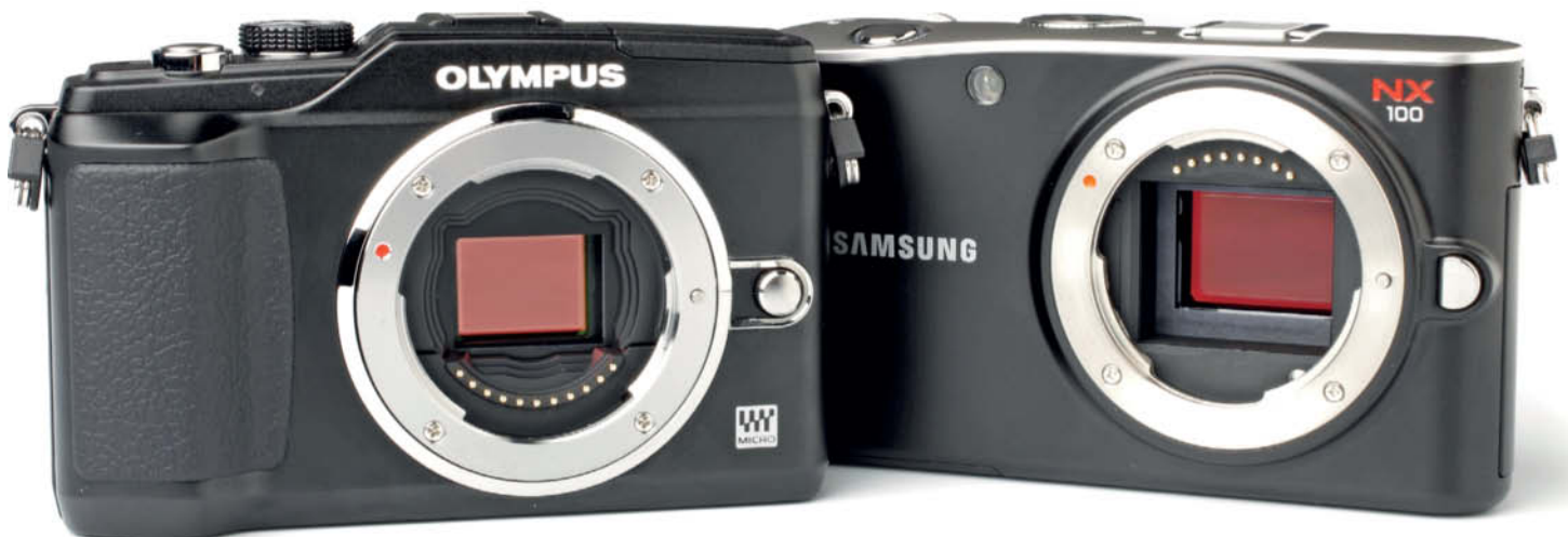
The Olympus Micro Four Thirds sensor (on the left) is approximately 40 percent smaller than the Samsung's APS-C model (on the right)
