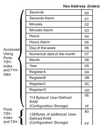
Figure 2. Real-Time-Clock Address Map
