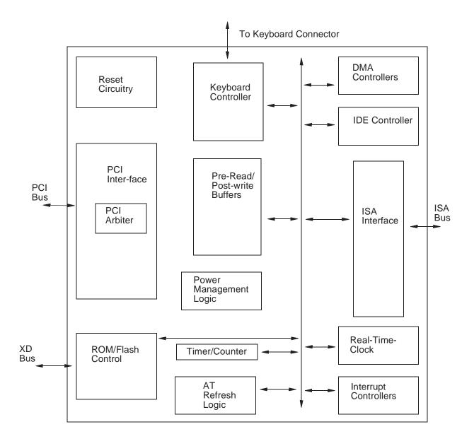
Figure 1. CY82C693 Functional Block Diagram
