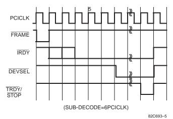
PCI Master Subtractive Decode "DEVSEL" Timing
